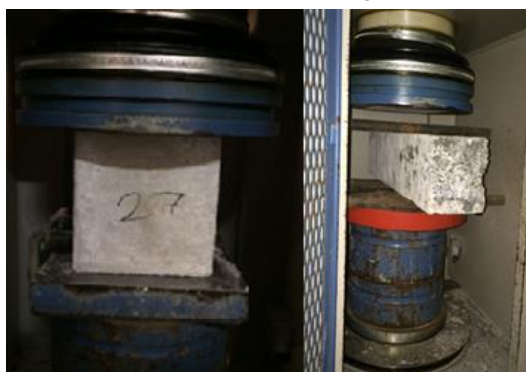
Fig. 1. Jack concrete crushing
