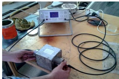
Fig. 3. Ultrasonic test (determining dynamic modulus of elasticity)
