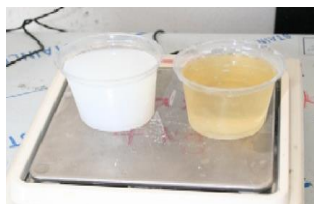
Fig. 2. Super plasticizer in the right hand and nano-silica in the left hand
